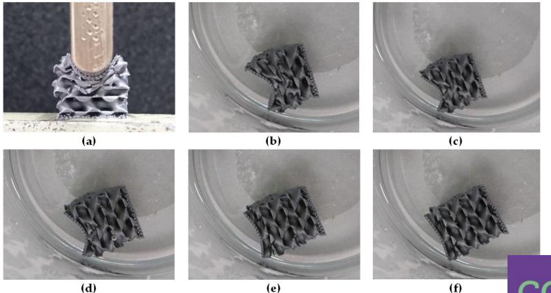
(a) Pressing sample G15 up to a maximum impact of 10 mm; (b)-(f) recovery process in water of 60  $^\circ\mathrm{C}$
