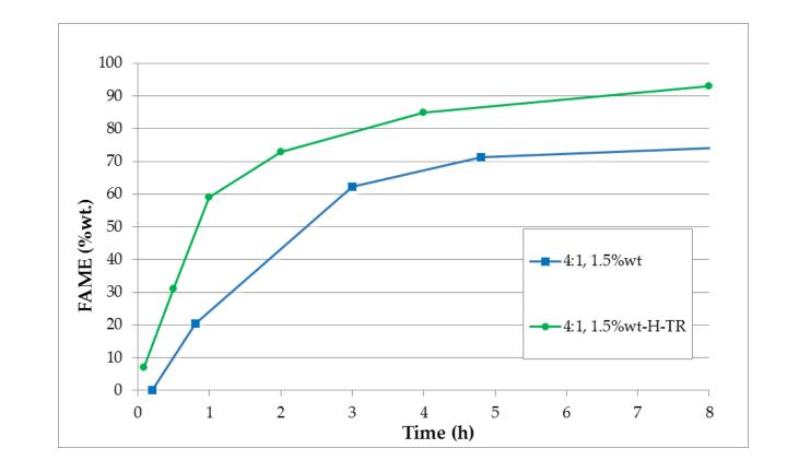
the high-throughput reactor is very promising, since both low temperature and methanol:oil molar ratio have been used
