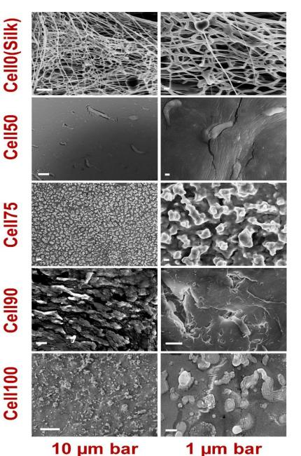
SEM analysis shows micro and nanomaterials after electrospinning procedure. From the images we found that Pure Silk can form homogeneous nanofiber matrices using EMIMAc IL generated films as the starting materials that are similar or better to silk fibers generated from organic solvent. As the cellulose content increases, the nanofiber structures gradually disappear and become more globular-like structures.
