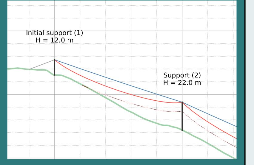
Skyline sag Measured in the middle of the span for four standard loads (7 to 35 kN) with a Vertex (instrument for foresters to measure height or distance)
