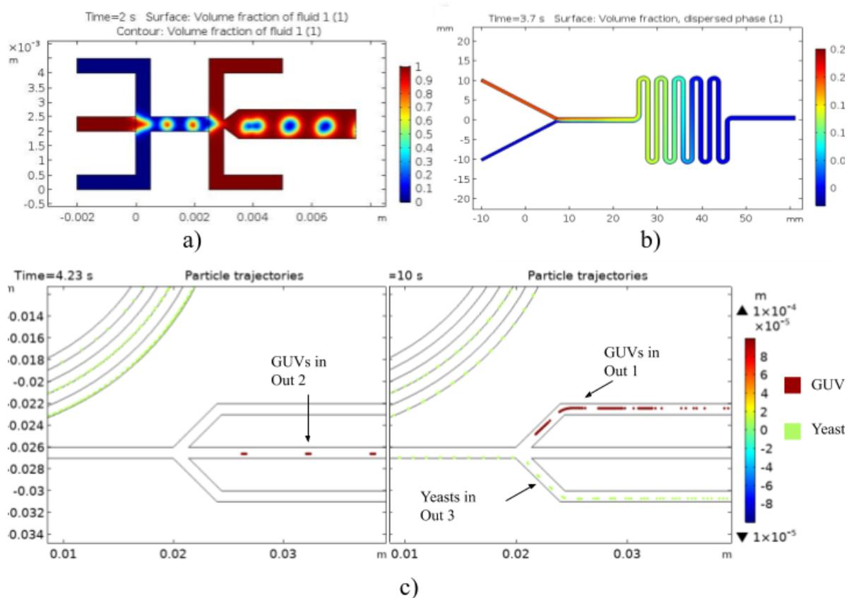
**Figure 2.** Multiphysics simulation results of the microfluidic system for (a) Volume fraction of double emulsions as templates for the synthesis of GUVs, (b) Volume fraction of the mixture model for the interaction between giant liposomes and translocating peptide expressing yeasts, and (c) Particles trajectories for the separation of loaded liposomes.
