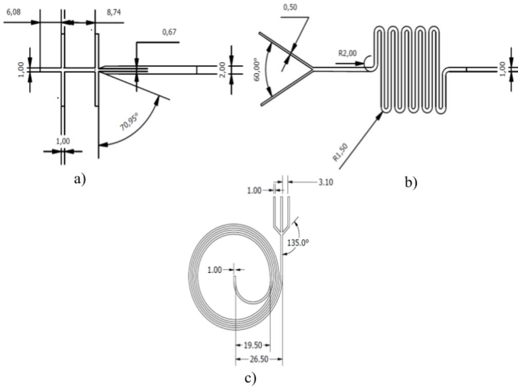
**Figure 1.** Design dimensions (mm) of the microsystems. (a) The WOW junction, (b) the Y-junction with a serpentine structure and (c) the inertial snail design.
