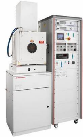
Magnetron sputtering system Auto 500 (BOC Edwards, England)
