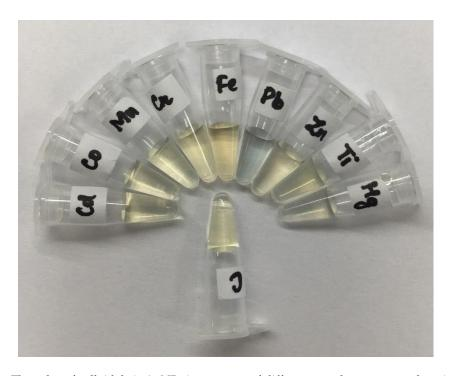
**Figure 4.** The color of colloidal cit-AgNPs in presence of different metals as compared to cit-AgNPs as control (C).
