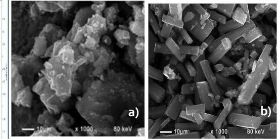
Figure 3. SEM images of lead citrate precursor synthesized by desulfurization and leaching of: a) a used PAM; b) a mixture of used PAM and NAM.
