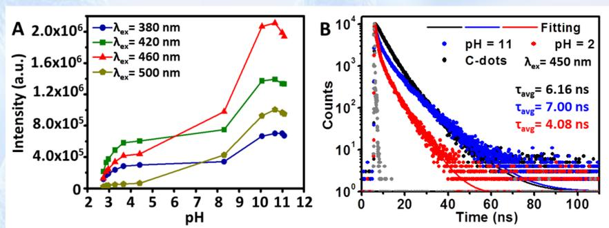
Figure 2. Plots presenting the pH dependence of PL intensity recorded at various excitation wavelengths (A) as well as PL lifetimes measured at  $\lambda_{ex} = 450$  nm (B) for C-dots aqueous dispersion.
