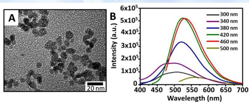
Figure 1. TEM image (A) together with the PL spectra of C-dots aqueous dispersion (B) recorded at excitation wavelengths ranging from 300 nm to 500 nm, with constant increment of 40 nm.
