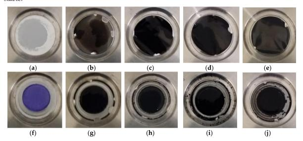
Figure 7. Filtration membranes: (a) CA substrate; (b) 40-ly rGO FM; (c) 60-ly rGO fm; (d) 80-ly rGO FM; (e) 100-ly rGO FM before permeation test; (f) CA substrate; (g) 40-ly rGO FM; (h) 60-ly rGO FM; (i) 80-ly rGO FM; (j) 100-ly rGO FM after permeation test.
