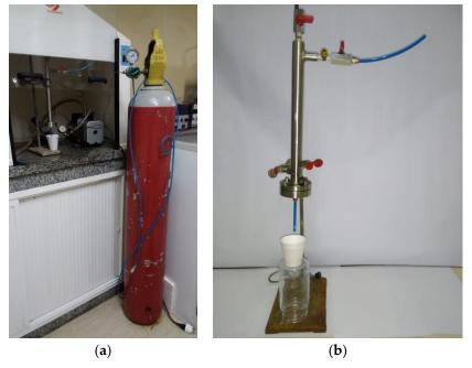
Figure 1. (a) Permeation system; (b) Permeation cell.
