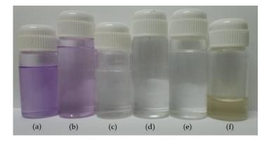
**Figure 9.** (a) feed solution; permeation solutions: (b) CA substrate; (c) 40-ly rGO FM; (d) 60-ly rGO FM; (e) 80-ly rGO FM; (f) 100-ly rGO FM.
