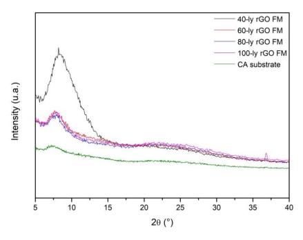
**Figure 4.** XRD patterns for CA substrate and rGO filtration membranes (FM) with different number of layers (ly).
