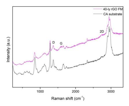
Figure 5. Raman spectra of CA substrate and 40-ly rGO FM.
