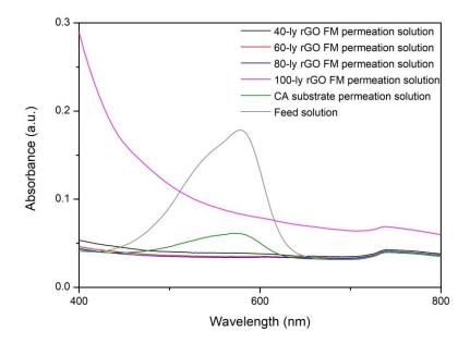
Figure 8. UV-vis absorption spectra for feed and permeation solutions.
