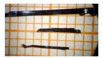
Fig. Photograph of  $WTe_2$  single crystals
