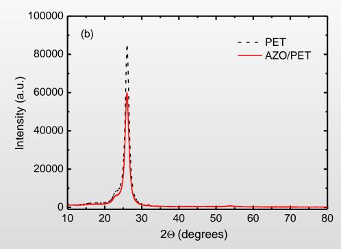
Figure: XRD of (a) AZO/mica and (b) AZO/PET structures
