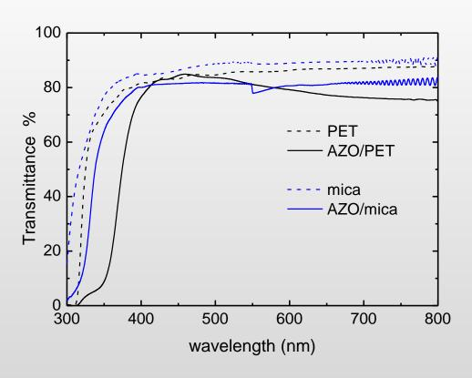
Figure: Transmittance spectra of AZO/mica and AZO/PET.
