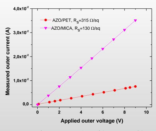
Figure: Ohmic behavior for AZO/mica and AZO/PET
