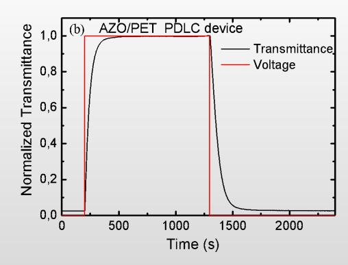
Figure: Response time of AZO/mica and AZO/PET PDLC devices
