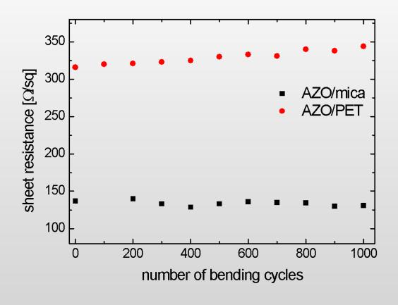
Figure: Sheet resistance dependence of the number of bending cycles for AZO/mica and AZO/PET
