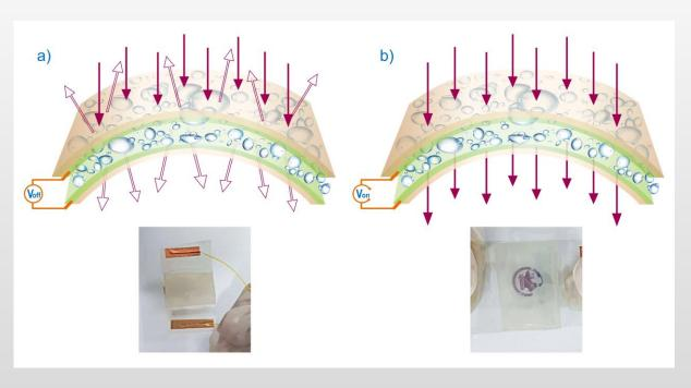
AZO/mica PDLC device at (a) "off" and (b) "on" states
