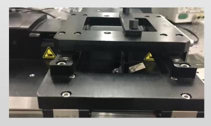
Bending test set-up
