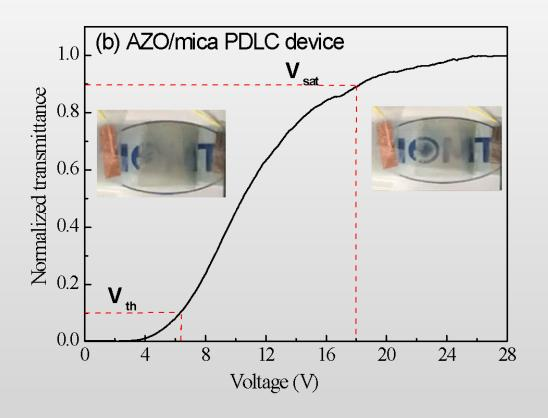
Figure: Voltage-transmittance curve and images at "off" and "on" states for AZO/mica and AZO/PET PDLC devices
