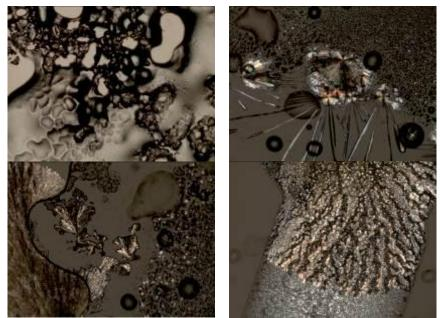
**Figure 6** Melting of CPL4 formulation (top left), followed by the onset of crystallization (top right and bottom left) and formation of crystalline dispersion (bottom right)
