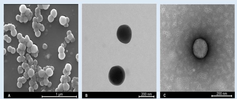
**Figure 1**. A) SEM visualization of MA SLNs, B) TEM micrographs without staining samples and C) with negative stained samples.
