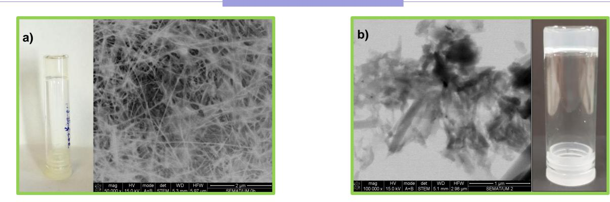
**Figure 3.** STEM images of hydrogels: a) Npx-Phe- $\Delta$ -PheOH (**7**) (0.4 wt%); b) Suc-Phe- $\Delta$ -PheOMe (**5**) (0.4 wt%).
