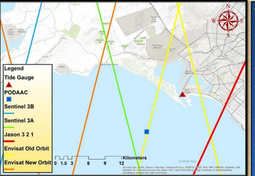
The location of the tide gauge station nearest to the study area. Multi-mission satellite tracks are also plotted in different colours representing the paths of Jason, Envisat (old and new orbits), and Sentinel A & B satellites. The nearest PODAAC grid to the Karachi gauge station can be visualized in Figure 3.
