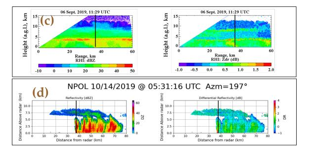
Vertical lines are at and above the disdrometers
