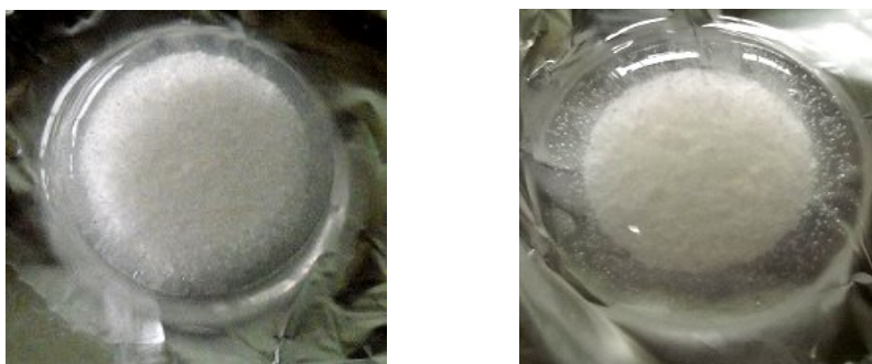
Figure 5. Photographs of different tablets prepared with Polyox ® WSR Coagulant as swelling testing progress
