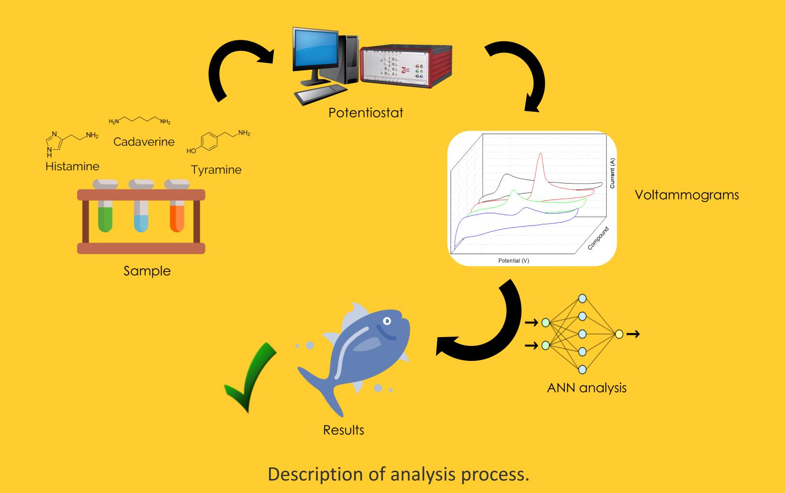
The final ANN structure had 51 input neurons, 5 neurons in the hidden layer, and 3 neurons in the output layer. The functions used for the hidden and output layers were *Tansig* and *Purelin*, respectively. The results show that this is a valid model with slopes near to 1 and intercepts close to 0. Moreover, it is important to remark that the worst correlation has a value of almost 0.900.
