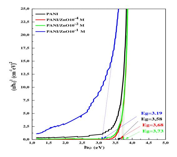
**Figure 7.** variation of  $(\alpha h\nu)^2$  as function of hv of PANI film and PANI/ZnO composite films electro polymerized at various concentrations of ZnO particles.
