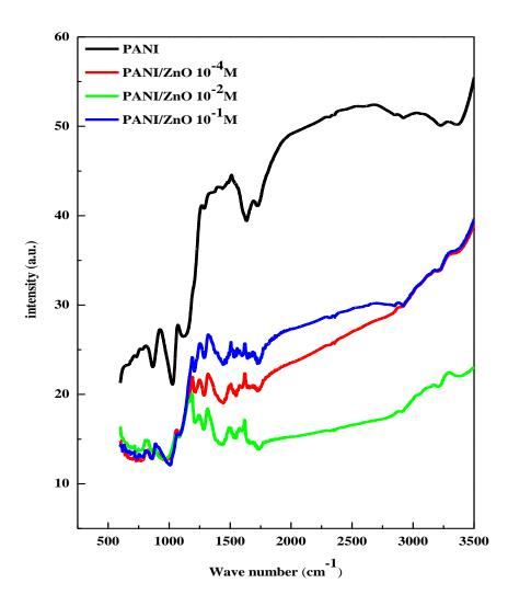
**Figure 8.** FTIR patterns of PANI and PANI/ZnO composite electropolymerized at differentes concentration of ZnO particle.
