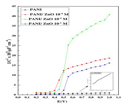
**Figure 3.** Mott schottky plot of PANI film and PANI/ZnO composite films electropolymerized at various concentrations of ZnO particles contact in 1M H<sub>2</sub>SO<sub>4</sub>+ 0.1M LiClO<sub>4</sub> with 500 Hz frequency.
