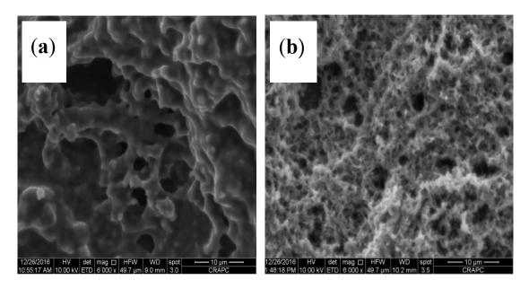
Figure 4. Scanning electron microscopy images: (a) PANI and (b) PANI/ZnO10<sup>-1</sup> M.
