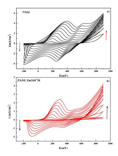
**Figure 1.** Electrochemical polymerization of: (**a**) ANI with 10 cycles, (**b**) ANI in presence of  $10^{-1}$  M ZnO with 10 cycles, in 1M H<sub>2</sub>SO<sub>4</sub>+10<sup>-1</sup>M LiClO<sub>4</sub>+10<sup>-1</sup>M ANI with scan rate of 10 mV/s.
