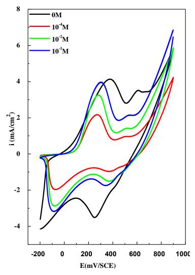
**Figure 2.** Cyclic voltammograms relating to the deposition of PANI and PANI/ ZnO composite film on ITO substrate in electrolyte containing 1M H<sub>2</sub>SO<sub>4</sub>+ 0.1M Aniline + 0.1M LiClO<sub>4</sub> with different concentration of ZnO particle in electrolyte at scan rate of 10 mV/s.
