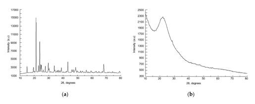
Figure 1. XRD patterns of: (a) SeO<sub>2</sub>; (b) SeO<sub>2</sub>/SiO<sub>2</sub>.
