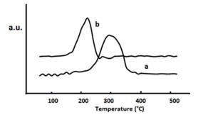
Figure 7. TPR profiles of: (a) SeO<sub>2</sub>/SiO<sub>2</sub>; (b) Pd/SeO<sub>2</sub>/SiO<sub>2</sub>.
