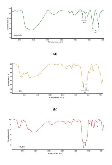
Figure 3. FTIR spectra of: (a) SeO<sub>2</sub>; (b) SiO<sub>2</sub>; (c) SeO<sub>2</sub>/SiO<sub>2</sub>.
