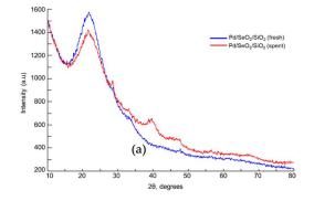
Figure 2. XRD pattern of: (a) fresh Pd/SeO<sub>2</sub>/SiO<sub>2</sub> catalyst; (b) spent Pd/SeO<sub>2</sub>/SiO<sub>2</sub> catalysts.
