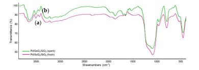
Figure 4. FTIR spectra of: (a) fresh Pd/SeO<sub>2</sub>/SiO<sub>2</sub>; (b) spent Pd/SeO<sub>2</sub>/SiO<sub>2</sub>.
