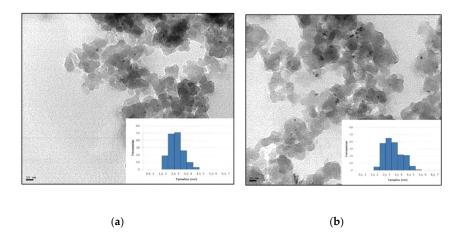
Figure 5. TEM images of: (a) fresh Pd/SeO<sub>2</sub>/SiO<sub>2</sub> catalysts; (b) spent Pd/SeO<sub>2</sub>/SiO<sub>2</sub> catalysts.
