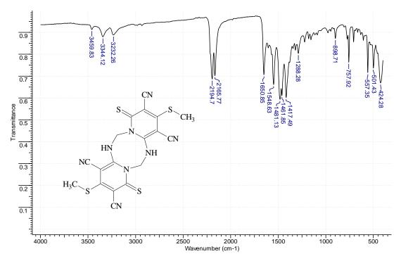
**Figure 2.** IR spectrum of 3,10-bis(methylthio)-1,8-dithioxo-5,6,12,13-tetrahydro-1H,8H-dipyrido[1,2-a;1',2'-e][1,3,5,7]tetrazocine-2,4,9,11-tetracarbonitrile (**4**; R = CH<sub>3</sub>, X = S).
