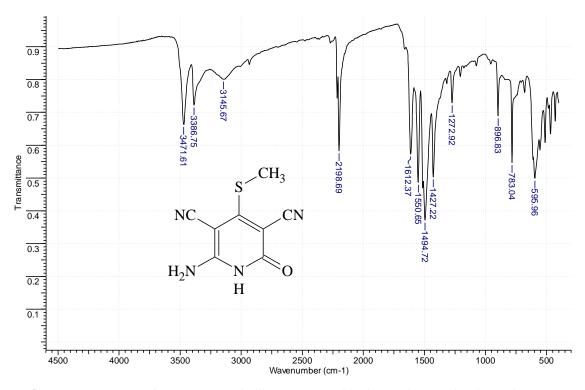
**Figure 1.** IR spectrum of 6-amino-4-(methylthio)-2-oxo-1,2 dihydropyridine-3,5-dicarbonitrile (**2**; R = CH<sub>3</sub>, X = O).
