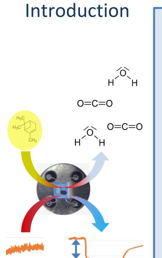
Semi conductor metal oxide sensors can detect volatile gases
