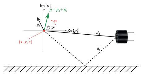
**Figure 4.** Direct (solid line) and reflected (dashed line) pressure components for a single transducer that are superimposed depending on the relative position of the transducer with respect to the reflecting surface, and total pressure generated by the transducer (green).
