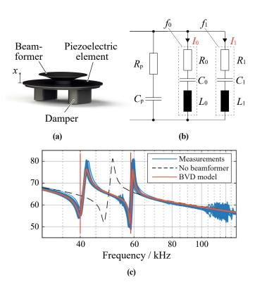
**Figure 3.** MSO-P1040H07T piezoelectric transducer: (a) Annotated rendering of the mechanical structure. (b) Electrical equivalent circuit diagramm BVD model showing the resonance paths at  $f_0 = 40 \, \text{kHz}$  and  $f_1 = 55 \, \text{kHz}$ . (c) Measured magnitude of the impedance and fitted BVD model.
