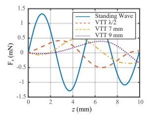
**Figure 7.** Vertical forces for a standing wave with a minimum at  $z = \lambda/4$ , and VTTs at  $z = \lambda/2$ , z = 7 mm, and z = 9 mm. The forces are obtained for an acoustically reflective surface at z = 0.
