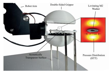
**Figure 1.** Double-sided gripper arrangement capable of picking objects with a density of  $> 7 \,\mathrm{g/cm^3}$  from acoustically transparent surfaces using a horizontal twin trap (HTT). The system is mounted to a robot arm for long-range movements.
