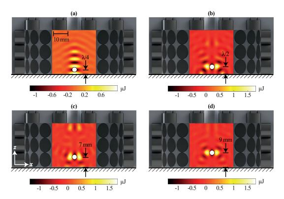
**Figure 6.** Force potential for (**a**) a standing wave with a minimum at  $z = \lambda/4$ , and VTTs at (**b**)  $z = \lambda/2$ , (**c**) z = 7 mm and (**d**) z = 9 mm. The potentials are obtained for an acoustically reflective surface at z = 0.
