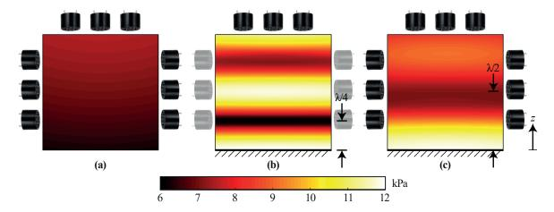
**Figure 5.** DMAP for (**a**) a single-sided array in free space, (**b**) the top part of the single-sided array with an acoustically reflecting surface at z=0 exhibiting high gradients that prohibit the generation of arbitrary focal points and (**c**) the single-sided arrangement with an acoustically reflecting surface at z=0 with a gradient that allows manipulation above a height of  $z=\lambda/4$ .
