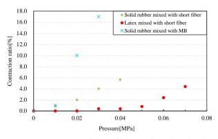
Figure 8. Contraction ratio of short-fiber-reinforced artificial muscle.
