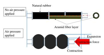
Figure 1. Straight-fiber-type artificial muscle.
