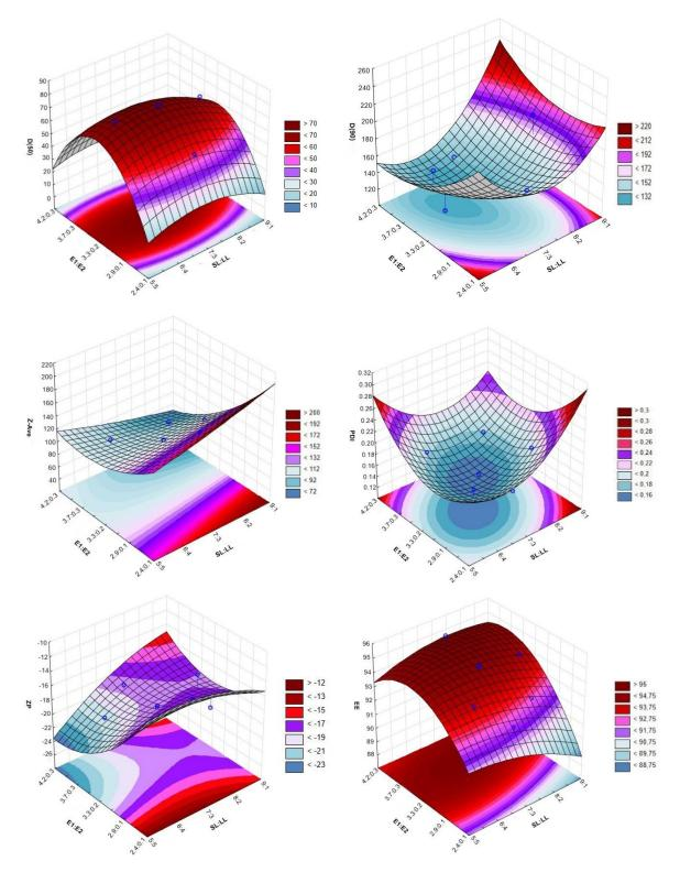
**Figure 2.** The 3-D surface plots portraying the effect of the ratio between the solid and liquid lipids (SL: LL) and the two emulsifiers (E1: E2) on the size (D(50): 50% of particles with size equal or lower to the given value, D(90): 90% of particles with size equal or lower to the given value and Z-Ave: mean particle size), polydispersity index (PDI), zeta potential (ZP) and encapsulation efficiency (EE)
