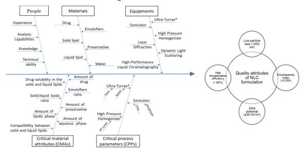
**Figure 1.** Ishikawa diagram showing the effects of critical material attributes (CMAs) and critical process parameters (CPPs) on critical quality attributes (CQAs), for the optimization of a NLC formulation.
