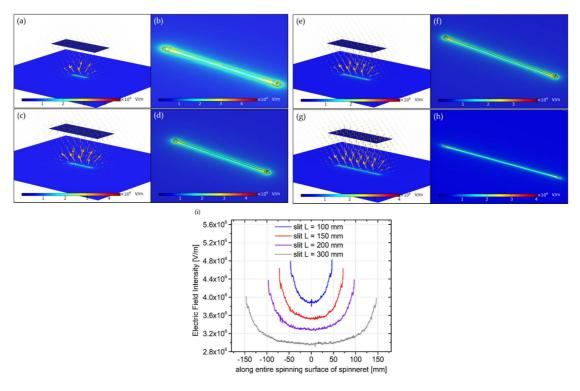
**Figure 5.** Electric field distribution depending on the slit length L: (**a**–**b**) L = 100 mm, (**c**–**d**) L = 150 mm, (**e**–**f**) L = 200 mm, (**g**–**h**) L = 300 mm, as well as its analytical verification along spinning surface of spinneret (**i**).
