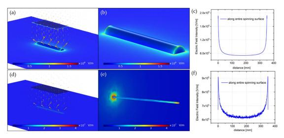
**Figure 2.** Electric field profile and its analytical verification of electrospinning systems: (a) cylinder and plate configuration, (b) E intensity near cylinder, (c) E strength along whole spinning surface, as well as (d) wire and plate arrangement, (e) E intensity near wire, (f) E magnitudes distributed along spinning surface of wire.
