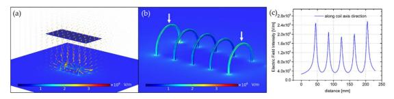
**Figure 4.** Simulated results of the spiral coil spinneret electric field profile: (a) spinning electrode-plate interaction, (b) spinneret electric field strength, (c) analysis of electric field distribution along coil axis direction.
