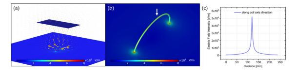
**Figure 3.** Electric field intensity simulated for the coil-plate electrospinning configuration: (a) electrostatic interaction between electrodes, (b) electric field strength of the spinneret and (c) analysis of the electric field distribution along coil axis direction.
