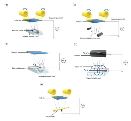
**Figure 1.** Schematic representation of the electrospinning configurations with spinnerets modeled and simulated in this paper: Nanospider Technology with (a) cylinder and (b) wire spinneret, (c) ring coil, (d) spiral coil, as well as (e) slit electrode.
