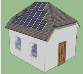
Figure 11 Angles Prevent Panels Filling a Hip Roof
