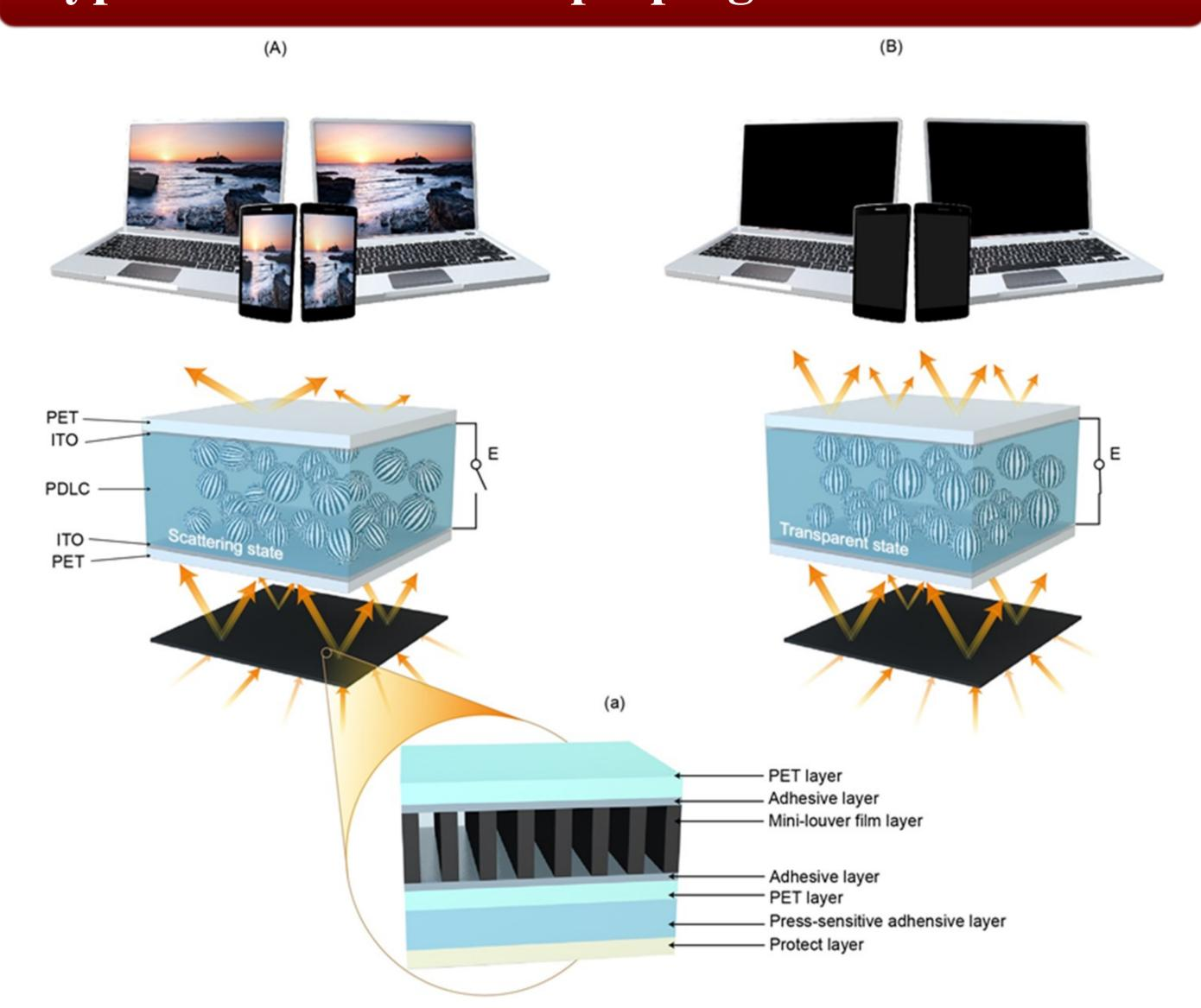
A novel switchable viewing angle film has been reported to make the viewing angle of an LCD electrically switchable between  $\pm$  30° and  $\pm$  60°.
