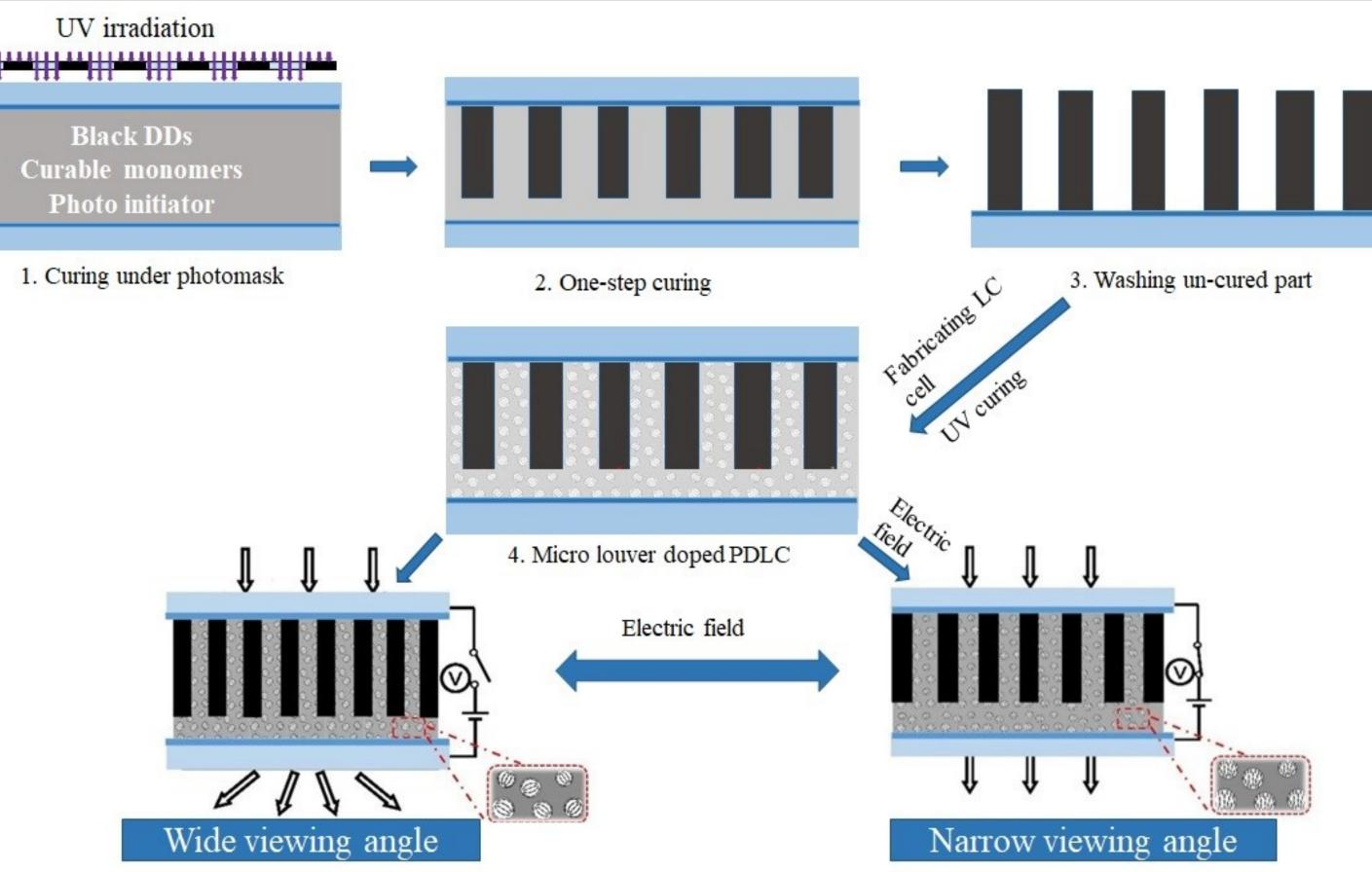
Here, we have developed an electrically switchable viewing angle device that fabricated by black dichroic dyes doped polymer dispersed cholesteric liquid crystals (DD-PSCLCs). By varying dimensions of the fabricated micro louver structures and voltages of electric field, view angle of the device can be tuned between wide viewing angle and narrow viewing angle.
