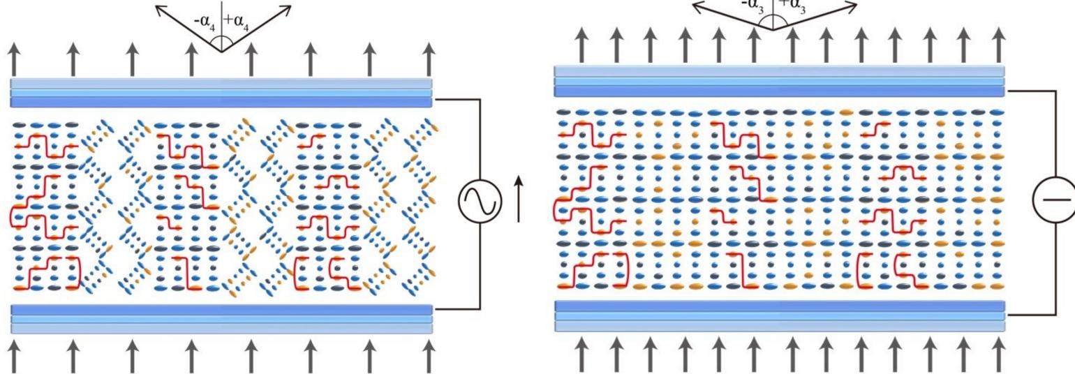
An electrically switchable viewing angle device that fabricated by dichroic dyes doped polymer stabilized cholesteric liquid crystals (DD-PSCLCs) has been developed.
