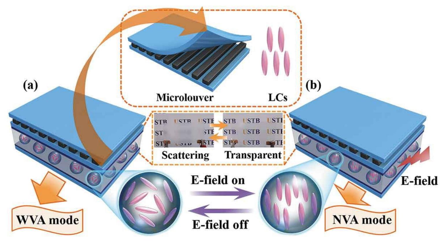
This work proposes a novel method for fabricating a controllable antipeeping device with a laminated structure of micro louver and a polymer dispersed liquid crystal (PDLC) film. the viewing angle ranges of the controllable anti-peeping device can be dynamically tuned by varying dimensions of the micro louver structures and applying various voltages across the PDLC film from 0 V to 8 V.
