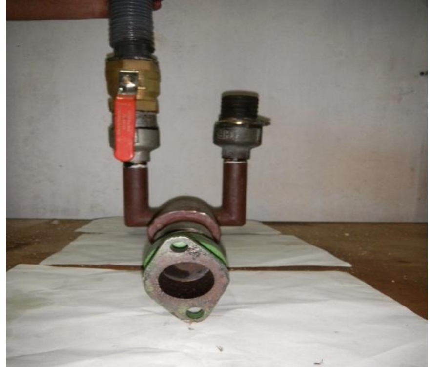
Fig. 6 Parallel flow gas entry carburetor
