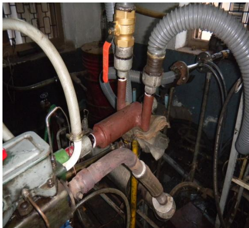
Fig. 4 Parallel gas entry carburetor for producer gas induction fitted to the engine
