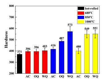
**Figure 4.** Hardness of different initial microstructures obtained by different austenitizing methods with as-received hot-rolled sample as comparison.
