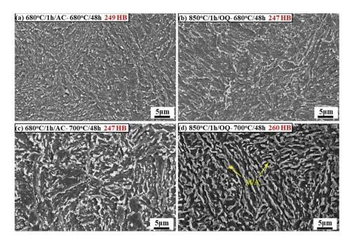
Figure 5. Microstructure of sample austenitized and then annealing: (a)  $680^{\circ}$ C/1h/AC- $680^{\circ}$ C/48h, (b)  $850^{\circ}$ C/1h/AC- $680^{\circ}$ C/48h, (c)  $680^{\circ}$ C/1h/AC- $700^{\circ}$ C/48h, (d)  $850^{\circ}$ C/1h/AC- $680^{\circ}$ C/48h.
