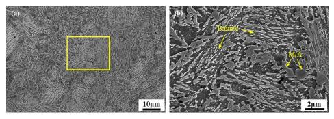
Figure 1. (a) SEM micrographs of hot-rolled sample; (b) Enlarged image of the yellow square in (a).
