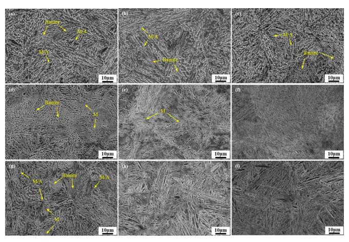
Figure 2. SEM micrographs of different initial microstructures obtained by different austenitizing process. (a)  $680 \, ^{\circ}\text{C/1h/AC}$ ; (b)  $680 \, ^{\circ}\text{C/1h/OQ}$ ; (c)  $680 \, ^{\circ}\text{C/1h/WQ}$ ; (d)  $850 \, ^{\circ}\text{C/1h/AC}$ ; (e)  $850 \, ^{\circ}\text{C/1h/OQ}$ ; (f)  $850 \, ^{\circ}\text{C/1h/WQ}$ ; (g)  $1000 \, ^{\circ}\text{C/1h/AC}$ ; (h)  $1000 \, ^{\circ}\text{C/1h/WQ}$ .
