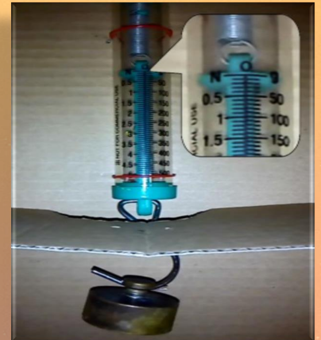
Spring scale measurement during free fall equaling 0N, 0g, while a 100g body is suspended from the spring's free endpoint.
