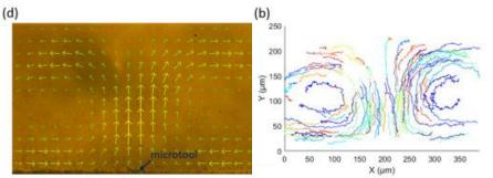
Natural flow convection observed in a microfluidic channel upon illuminating the gold-coated disk of a single microswimmer. Such localized micromixing can be highly beneficial for lab-on-a-chip biosensing applications.
