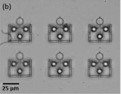
Disk microswimmers for thermoplasmonic mixing 3D printed without (left) and with (right) a mask allowing for subsequent selective gold coating of the disk.
