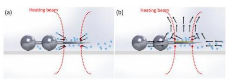
Schematic of the flow effect induced by microswimmers without (left) and with (right) gold coating of the disk area.
