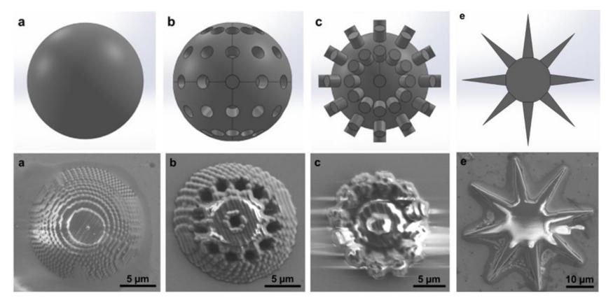
3D designs (top) and scanning electron micrographs (bottom) of spherical microswimmers for drug delivery studies involving the mucus biobarrier. The microswimmers were fabricated in the IP-L 780 polyacrylate resin by two-photon polymerization on a Nanoscribe GT. The various features are meant to increase the surface area, allow loading with drugs or excipients, as well as increase penetration through mucus.
