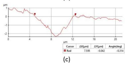
**Fig.6** Wear scratch on dental material – CHARISMA 40" under a force of 100µN:
