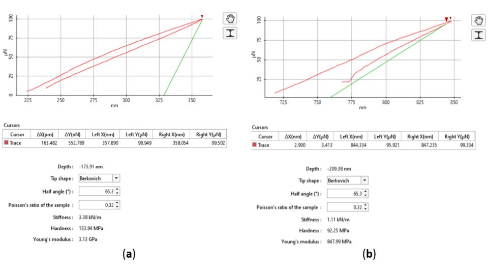
**Fig.4** Nanoindentation curves of dental material – CHARISMA 40" under a force of 100  $\mu$ N at: (a) 20°C, (b) 100 °C
