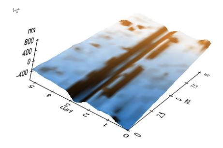
**Fig.5** Wear scratch on human teeth under a force of 100µN:
