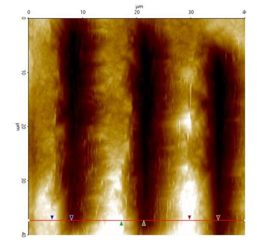
Fig.7 Wear scratch variation of dental material – CHARISMA 40" under a force of  $100\mu N$  for different temperatures
