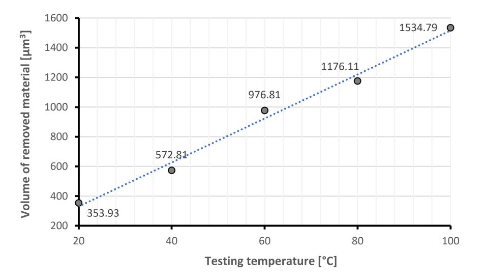
**Fig.9** Wear volume variation of dental material – CHARISMA 40" for different temperatures under a scratching forces F=100µN
