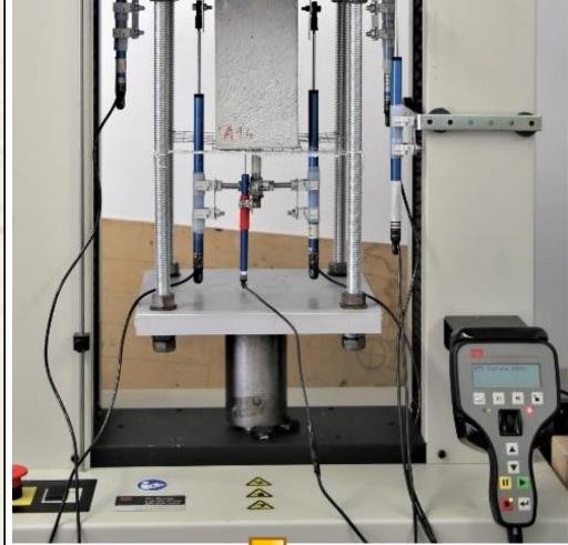
Each specimen was instrumented with 5 Potentiometric Linear **Transducers (PLT):**
