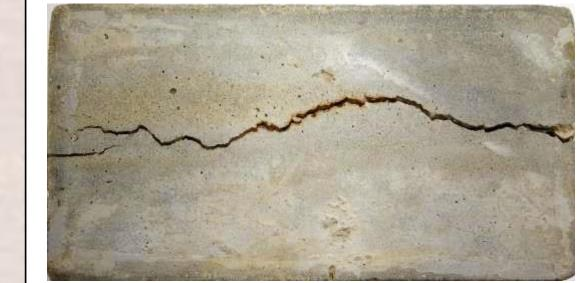
Through the use of a digital microscope, it was possible to accurately detect each crack width and then calculate the average of all sides.
