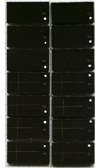
Cathodic dip-paint lacquering (KTL)
