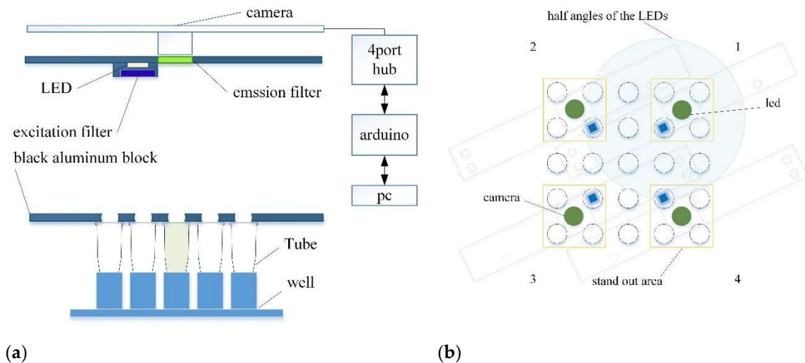
**Figure 1.** (a) System structure diagram (b) 4 quadrants of all  $5 \times 5$  wells: camera and LED location.
