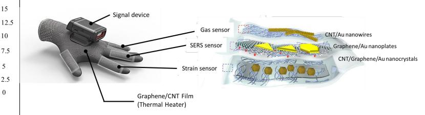
Based on the flexible substrates of graphene and carbon nanotubes and different structures of gold nanocrystals, it's expected to be applied to different types of wearable flexible sensors, such as gas sensors, strain sensors and SERS sensors, etc.
