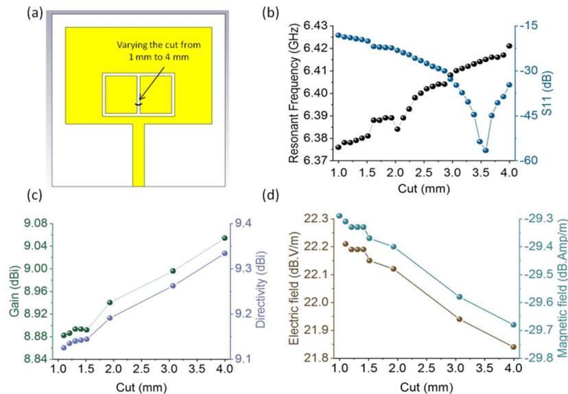
**Figure 2.** CST Simulations: (a) Front view of the design, (b) The change in resonant frequency and corresponding maximum S11 response, (c) Maximum Gain and Directivity, (d) Maximum electric field and magnetic field by varying the cut from 1 to 4 mm as shown the above patch shown in Figure 1d(iii)).
