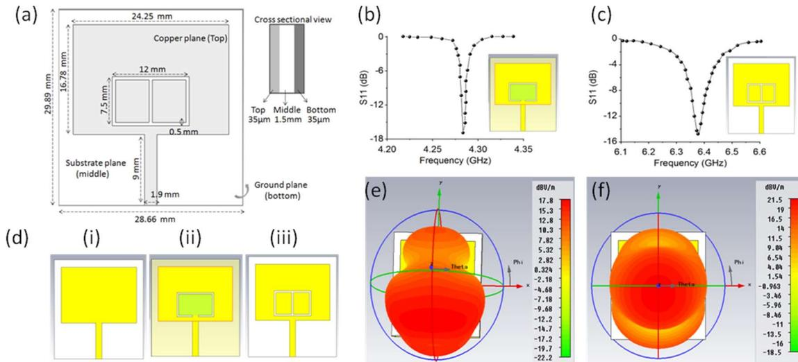
**Figure 1.** (a) Design parameters of patch antenna. (b-c) S11 response of patch shown in inset. (d) (i) initial design of patch, (ii) improvement in the initial design, (iii) final design. (e-f) electric field corresponding to patch d(ii) and d(iii) respectively.
