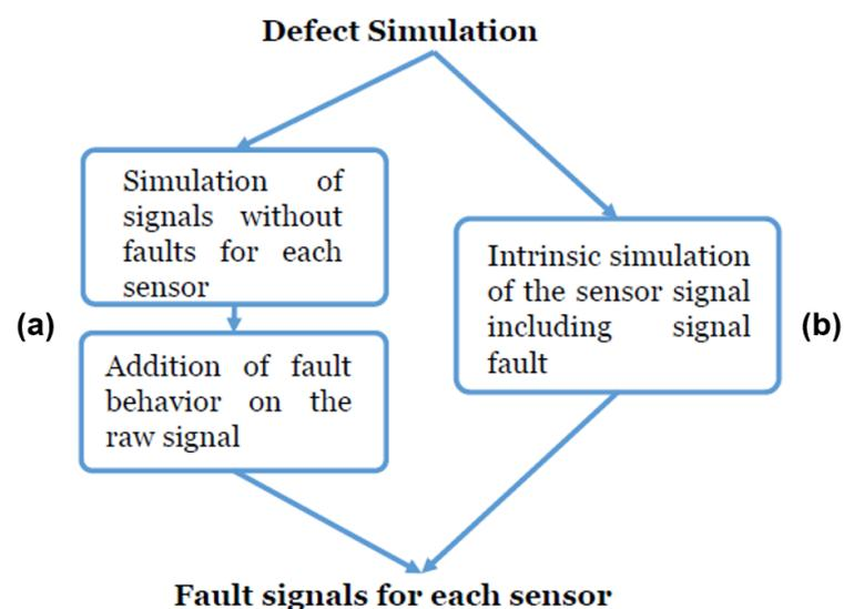
**Figure 3.** Different Approaches for the Sensor Fault Model. (a) shows a post-simulation approach, where the faults are added after the sensor signal was simulated by the Sensor Response Model. (b) shows the intrinsic simulation approach, where the fault behavior is integrated in the Sensor Response Model.
