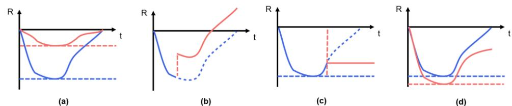
**Figure 1.** Different examples of defects (original signal in blue, defect in red). (a) Sensitivity Loss leading to a lower resistance response to a gas concentration. (b) Signal Jump causing an abrupt additive change in the signal. (c) Sensor Stopping leading to constant sensor outputs and (d) Battery Loss causing a lower heating temperature, which leads to a slower sensor recovery process.
