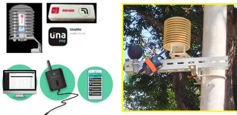
**Figure 3.** UnaSense (left up) and Temphawk (left down) sensors and the installation.
