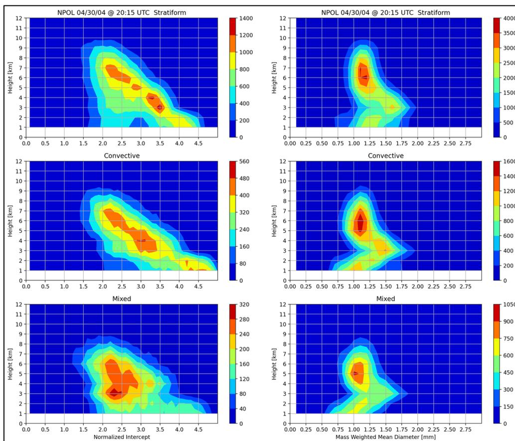
Figure 5. 2D histograms of  $N_w$  (left panels) and  $D_m$  (right-panels) as a function of height [km], for stratiform rain (top panels), convective rain (middle panels) and mixed (bottom panels).
