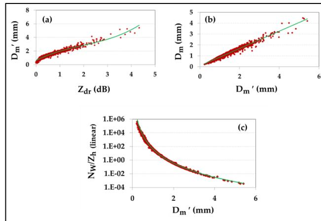
Figure 1. S-band simulation results of (a)  $D_m'$  versus  $Z_{dr}$ ; (b)  $D_m$  with  $D_m'$ ; (c)  $N_w/Z_h$  (linear) versus  $D_m'$ .
