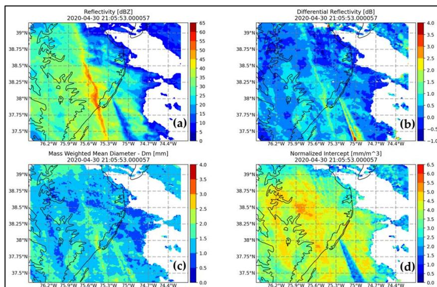
Figure 2. NPOL gridded data at 1000 m altitude with 500 m by 500 m pixel resolution; (a)  $Z_h$ ; (b)  $Z_{dr}$ ; (c) estimated  $D_m$ ; (d) estimated  $N_w$ .
