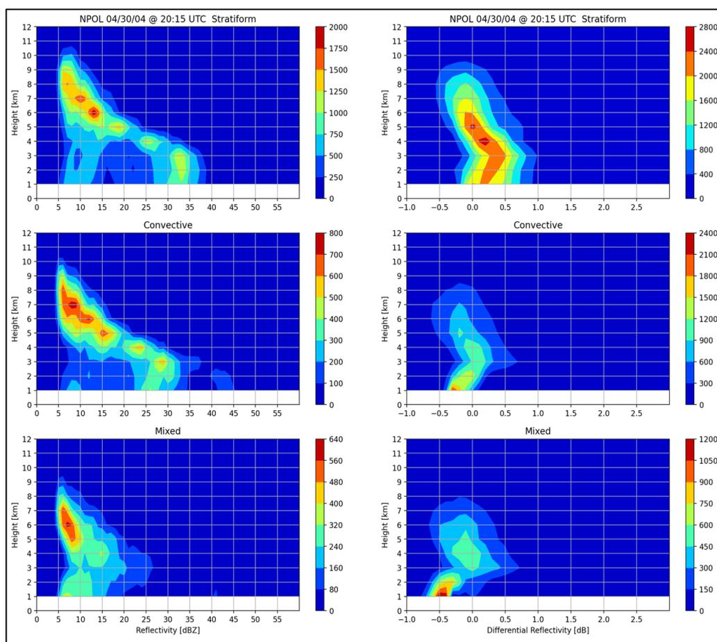
**Figure 4.** 2D histograms of Reflectivity (left panels) and Differential Reflectivity (right-panels) as a function of height [km], for stratiform rain (top panels), convective rain (middle panels) and mixed (bottom panels).
