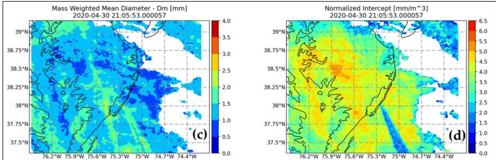
The gridded data ranging from -60 km to +60 km both in the North-South and the East-West directions were extracted and the classification based on the  $N_W$  -  $D_m$  values for each pixel was determined.
