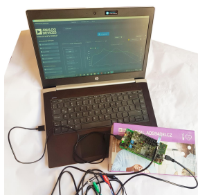
Figure 2. Integrated electronic tongue system. Computer with Sensor Pal software, USB cable to the EVAL-AD5940ELCZ and EVAL-ADICUP3029 attached boards, colored crocodile cable, sensor connection cable and SPE Sensor.
