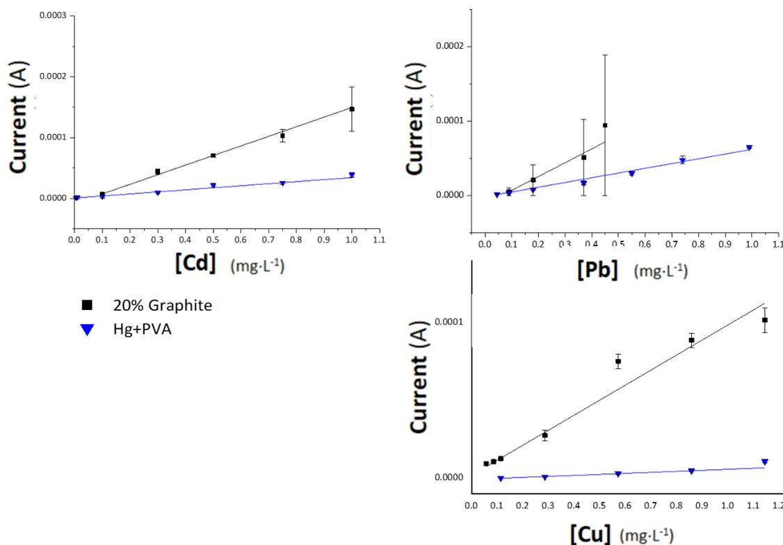
**Figure 4.** Calibration curves for Cd (a), Pb (b) and Cu (c) for 20% graphite (black) and 20% graphite plus Hg-NPs (blue).
