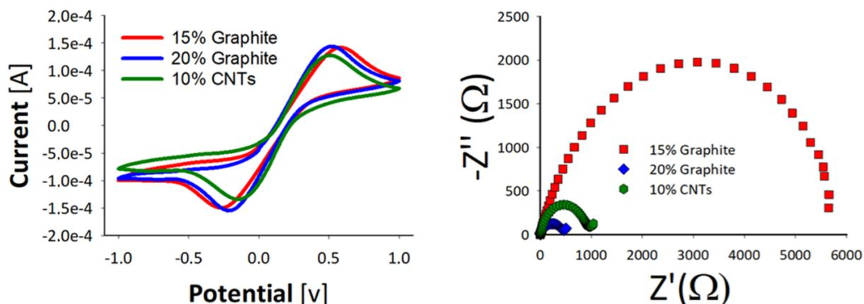
Figure 1. CV (a) and EIS (b) characterization of the different electrodes.
