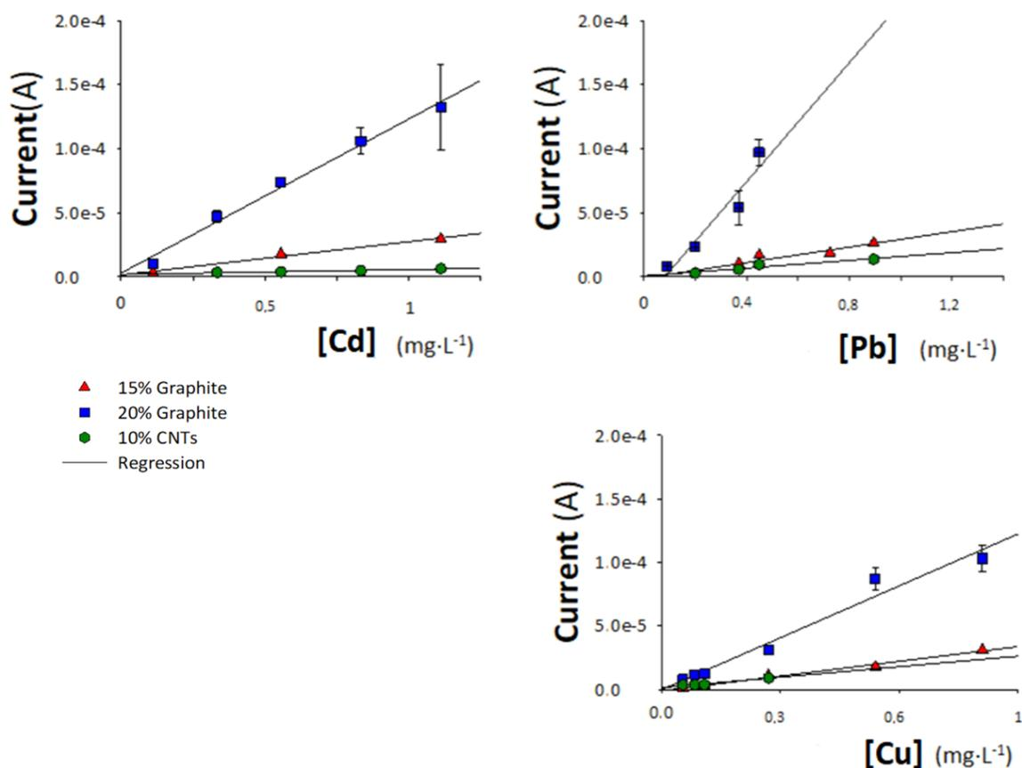
Figure 3. Calibration curves for Cd, Pb and Cu for each raw material.
