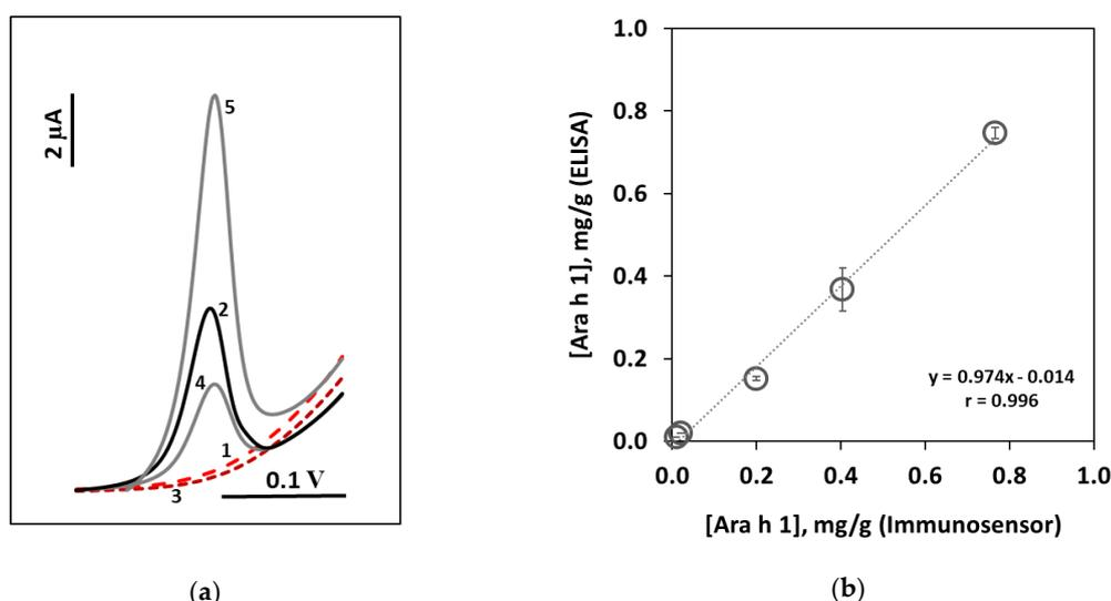
**Figure 2.** Analysis of food products. (a) LSV voltammograms (solid lines – presence of Ara h 1; dashed lines – absence of Ara h 1); (b) Correlation between the obtained results for the analysis of food products using the developed immunosensor and the commercial ELISA kit. (1) Cereal bar (no peanut), (2) Energy bar containing peanut, (3) Cookie that "may contain peanut", (4) Granola that "may contain peanut", (5) Pineapple cookie containing 8% of peanut.
