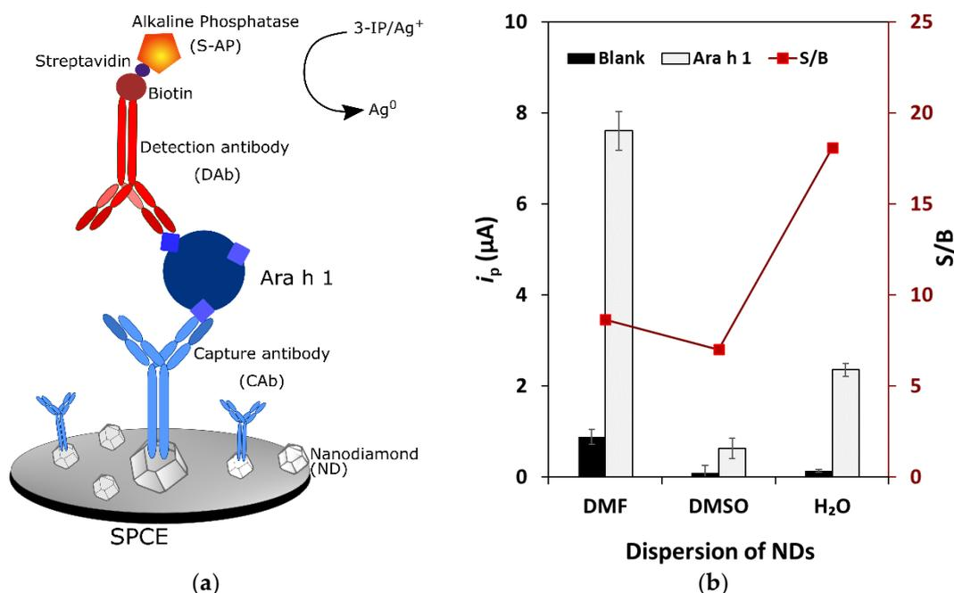
**Figure 1.** Nanodiamond-based voltammetric immunosensor. (a) Schematic representation of the immunosensor construction; (b) Results obtained for NDs 1 mg/mL dispersed in DMF, DMSO and H<sub>2</sub>O. Experimental parameters: CAb 10 μg/mL, Ara h 1 (0 and 250 ng/mL), DAb 250× dilution, S-AP 200,000× dilution, 3-IP (1.0×10<sup>-3</sup> M), Ag<sup>+</sup> (4.0×10<sup>-4</sup> M).
