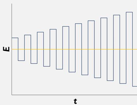
The potential modulation of  $E_{sw}$ -EFS consists of SW forward and reverse potential pulses of constant frequency imposed on a constant mid-potential. The duration of potential cycles is constant but the height of the pulses (i.e. amplitude) progressively increases.
