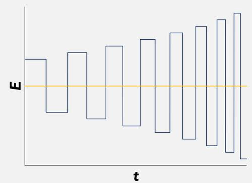
The technique called multi-EFS was created by combination of f-EFS and  $E_{sw}$ -EFS. The duration of potential cycles progressively decreases. At the same time, the amplitude of pulses for the following cycles gradually increases.
