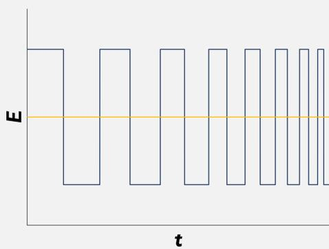
The potential modulation of technique called f-EFS consists of SW forward and reverse potential pulses imposed on a constant mid-potential. The duration of potential cycles progressively decreases (i.e. the frequency increases during the experiment).
