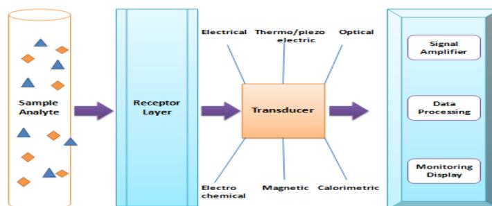
**Figure 1.** Schematics of a biosensor unit.
