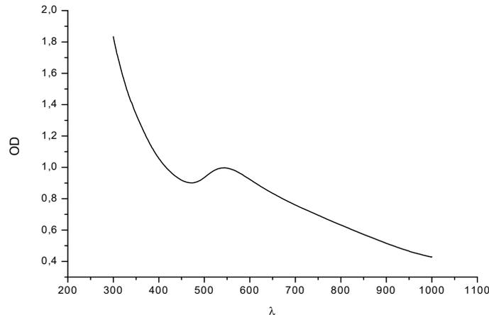
*Absorption spectra of Au nanoparticles embedded in glycan matrix*
