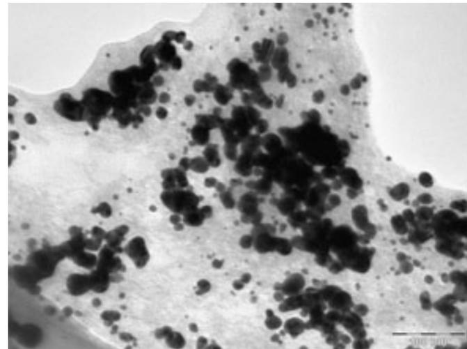
*TEM image of Au nanoparticles embedded in glycan matrix*
