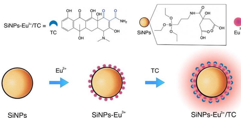
**Scheme 1.** Schematic illustration the design of luminescent SiNPs- $\text{Eu}^{3+}$  nanoprobe for tetracycline (TC) detection.
