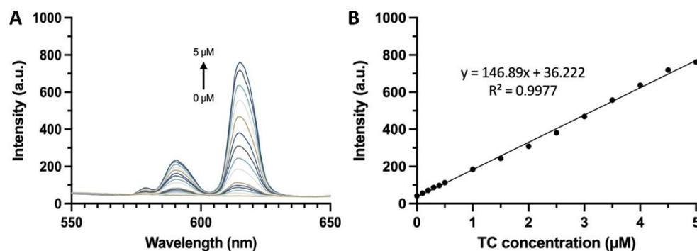
**Figure 3.** Luminescence response of SiNPs-Eu<sup>3+</sup> nanoprobe to TC in 50 mM Tris-HCl buffer of pH 8.5. (A) Emission spectrum of 1 mg/mL SiNPs-Eu<sup>3+</sup> nanoprobe in the presence of different concentration of TC (concentrations are 0, 0.1, 0.2, 0.3, 0.4, 0.5, 1.0, 1.5, 2.0, 2.5, 3.0, 3.5, 4.0, 4.5, and 5.0  $\mu$ M). (B) Emission intensities at 615 nm of SiNPs-Eu<sup>3+</sup> nanoprobe against the concentrations of TC.
