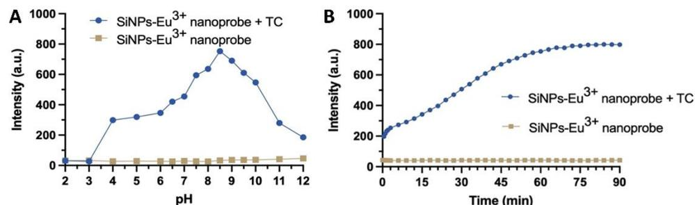
**Figure 2.** Emission intensities at 615 nm of SiNPs-Eu<sup>3+</sup>/TC samples at different (A) pH condition and (B) time point. (A) Luminescence intensity of 1 mg/mL SiNPs-Eu<sup>3+</sup> nanoprobe in the presence and absence of 5  $\mu$ M TC in 50 mM Tris-HCl buffer of different pH. (B) Time-dependent luminescence response of 1 mg/mL SiNPs-Eu<sup>3+</sup> nanoprobe to 0 and 5  $\mu$ M TC in 50 mM Tris-HCl buffer of pH 8.5, respectively.
