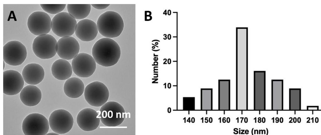
**Figure 1.** Characterization of SiNPs-Eu<sup>3+</sup> nanoprobe. TEM image (A) and size distribution (B) of SiNPs-Eu<sup>3+</sup> nanoprobe.
